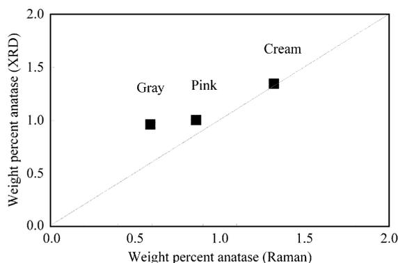
Fig. 6. Raman versus XRD results for quantification of anatase in the HG (gray kaolin), HP (pink kaolin), and HC (cream kaolin) series. The 1:1 slope line is presented for reference.
