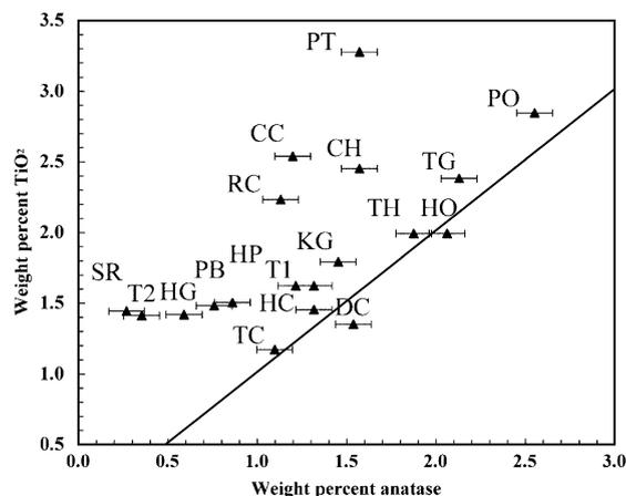
Fig. 7. Weight percent total  $\text{TiO}_2$  (measured by XRF) versus weight percent anatase (measured by Raman) for commercial kaolins. Bars represent average standard errors for each method. The 1:1 slope line is presented for reference. See Table 1 for ID codes.
