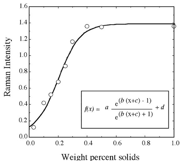
Fig. 1. Raman intensity at 144  $\text{cm}^{-1}$  plotted as a function of percent solids in a kaolin slurry. Concentration of anatase in dry kaolin is approximately 1 wt.%. Data collected with 256 scans and laser power = 0.05 W. The line represents a least-squares optimization using a sigmoid function (Raner, 1998). Coefficients corresponding to the best fit are  $a=0.67$ ,  $b=13.2$ ,  $c=-0.20$ , and  $d=-0.72$ .
