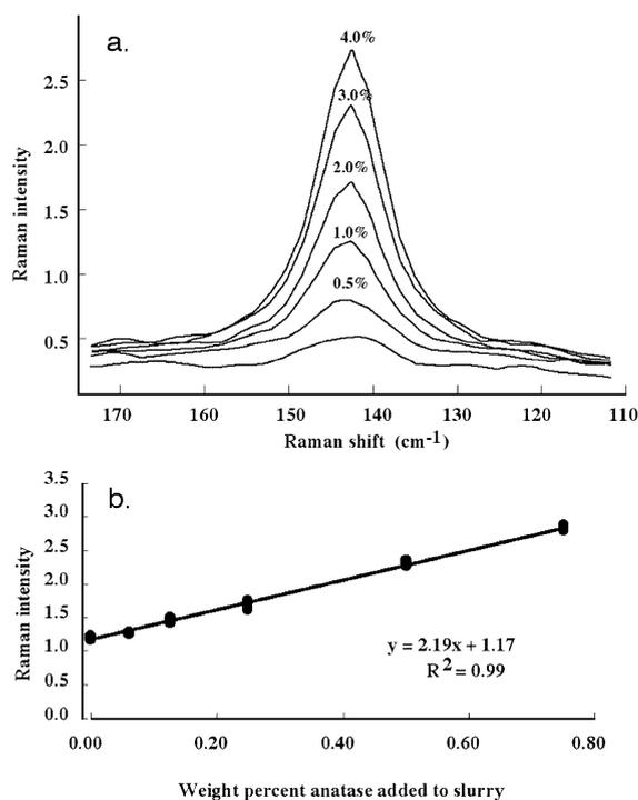
Fig. 2. (a) Raman spectra showing  $144\text{ cm}^{-1}$  peak of slurries sample with standard additions ranging from 0 to 4 wt.% anatase. Data collected with 256 scans, laser power = 0.125 W, and background correction. (b) Raman intensity at  $144\text{ cm}^{-1}$  plotted as a function of weight percent synthetic anatase added to anatase-bearing kaolin slurry. Using the internal standard method of Skoog et al. (1998), the sample contains  $2.1 \pm 0.1$  wt.% anatase.
